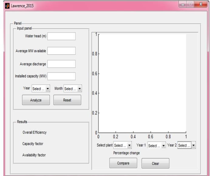
Figure 3. Graphical User Interface Model for Performance Parameters using Matlab
