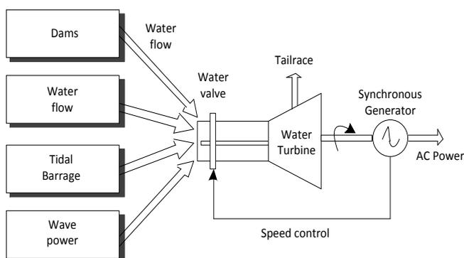
Figure 1. Hydro Electric Generation
