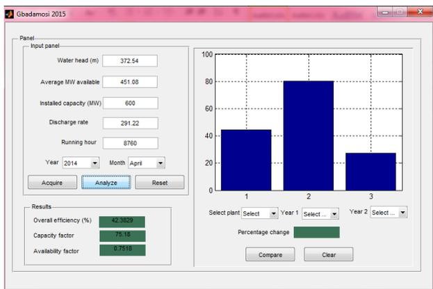
Figure 9. GUI Model Comparing the Average, Highest & Lowest Plant Overall Efficiencies
