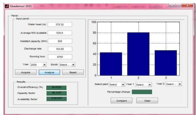
Figure 7. GUI Model Comparing the Plant Overall Efficiencies of 2004, 2005 & 2006
