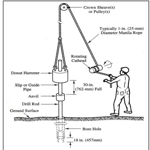
Figure 3. Standard Penetration Test Arrangements
