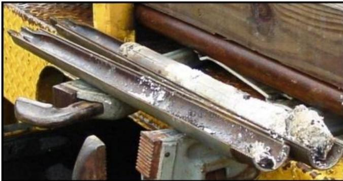
Figure 1. Split Spoon Sampler used in SPT
