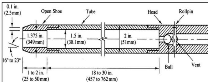
Figure 2. Standard dimensions for the SPT sampler
