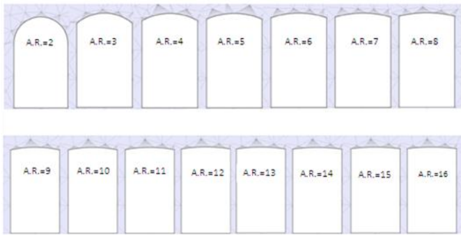
Fig. 6. The modeling of vaulted tunnels with width of 4 meters and different arch radius (A.R. is arch radius of tunnel to meter)
