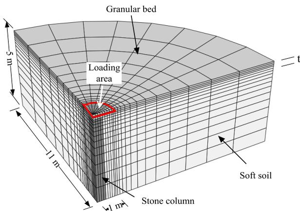
Figure 1. Typical mesh shape for numerical analyses
