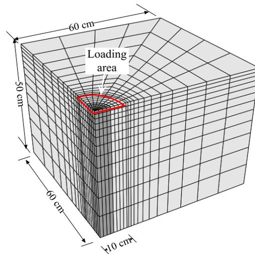
Figure 2. Mesh discretization of model tests by [18]
