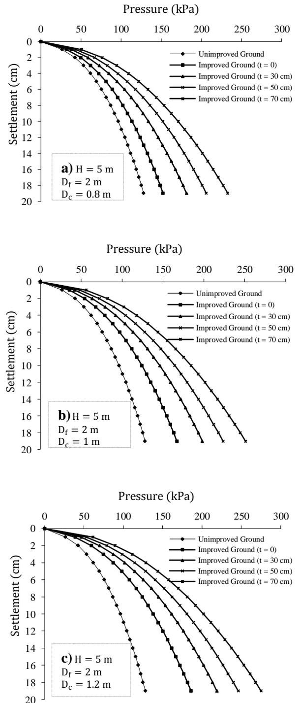
Figure 4. Pressure versus settlement curves for different diameters of stone columns: a)  $D_c = 0.8$  m, b)  $D_c = 1$  m, c)  $D_c = 1.2$
