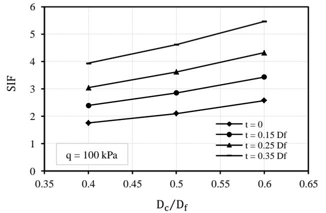
Figure 6. SIF versus the  $D_c/D_f$  for different thickness of granular bed at pressure of 100 kPa
