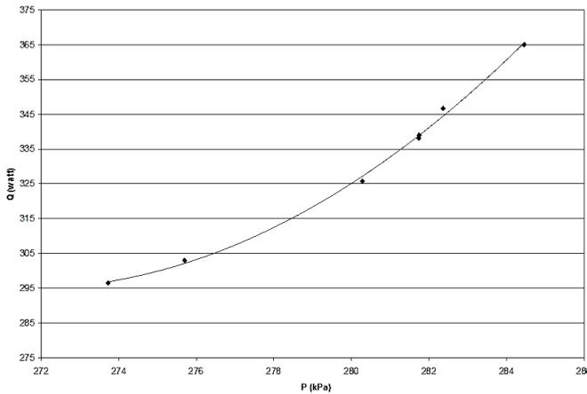
Figure 8. Variations of axial heat flux changes with saturation pressure for steady state in temperature interval 129.5- 131°C
