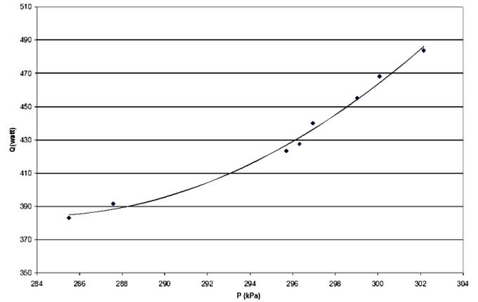
Figure 9. Variations of axial heat flux changes with saturation pressure for steady state in temperature interval 131-133.5°C
