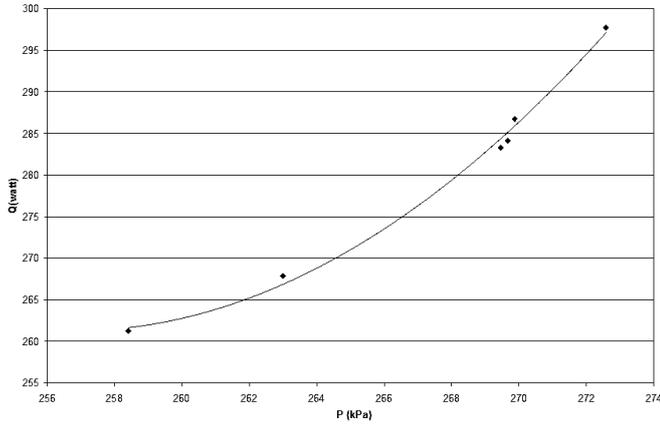
Figure 7. Variations of axial heat flux changes with saturation pressure for steady state in temperature interval 127.5- 129°C
