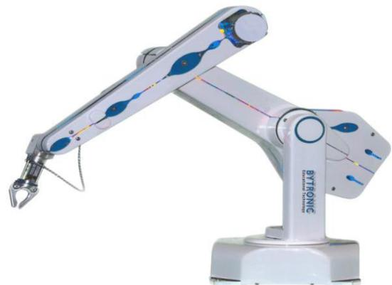
Figure 4. 5 Axis Robotic Arm
