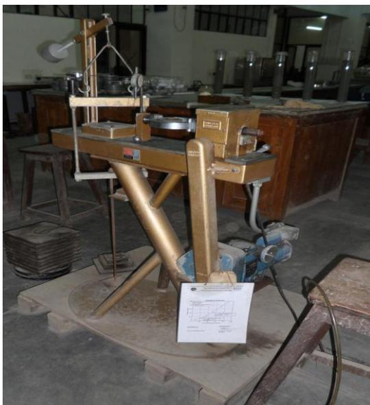
Fig. 4: Laboratory preparation for direct shear test.
