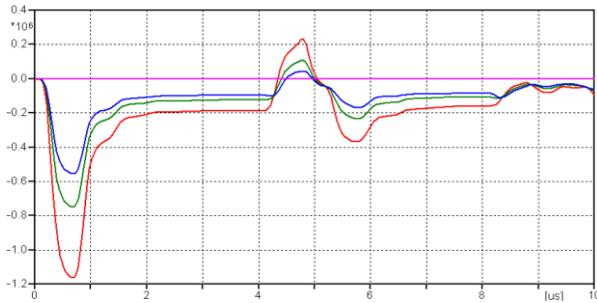
Figure 19. Range of excess voltage generated in phases of the extended line model
