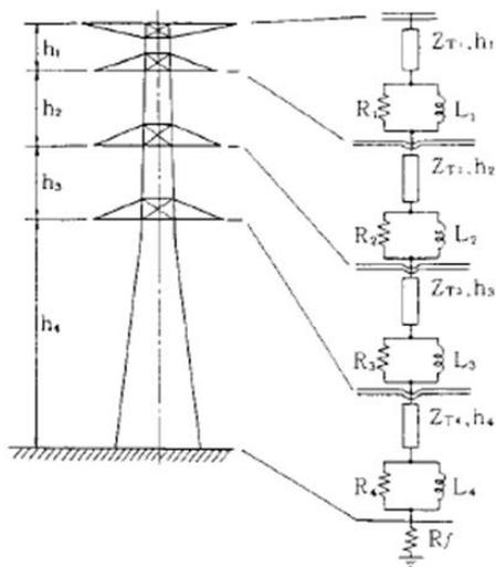
Figure 2. The multistory model of a tower
