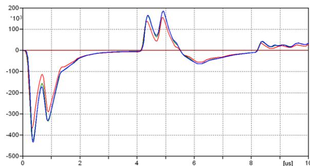
Figure 14. Range of the voltage generated on both ends of insulators in the multistory model
