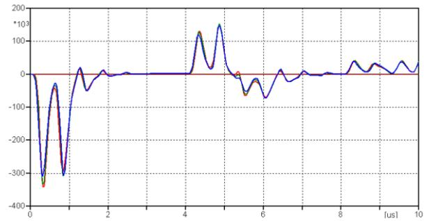
Figure 15. Range of the voltage generated on both ends of insulators in the simplified multistory model
