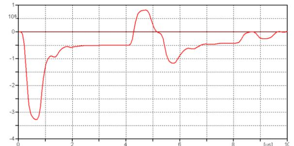
Figure 9. Range of the generated voltage in the place of thunder strike surge in the simplified multistory model
