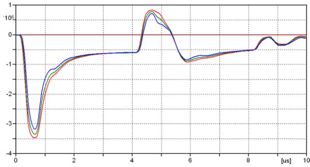
Figure 11. Voltage range created in tower arms relative to the ground in the multistory model
