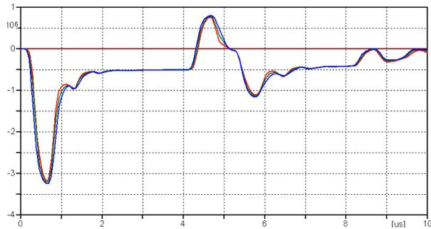
Figure 12. Voltage range created in tower arms relative to the ground in the simplified multistory model
