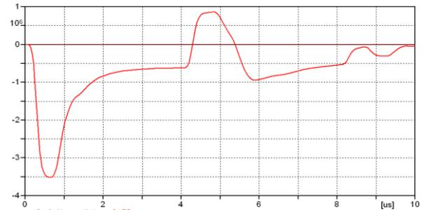
Figure 8. Range of the generated voltage in the place of thunder strike surge in the multistory model
