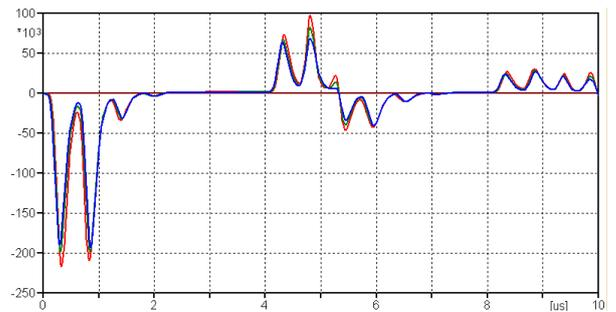
Figure 16. Range of the voltage generated on both ends of insulators in the simplified extended line model
