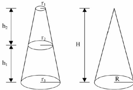
Figure 5. Tower equivalent structure
