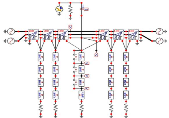
Figure 4. The simplified multistory equivalent circuit
