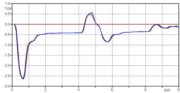
Figure 13. Voltage range created in tower arms relative to the ground in the simplified extended line model
