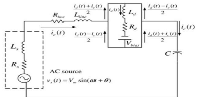
Figure 5. Circuit diagram of the CETL in the steady state with its initial transient when  $i_d$  is equal to or higher than the peak of  $i_c$ .
