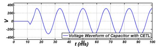
Figure 14. The voltage waveforms of capacitor with limiter and angle 0°.
