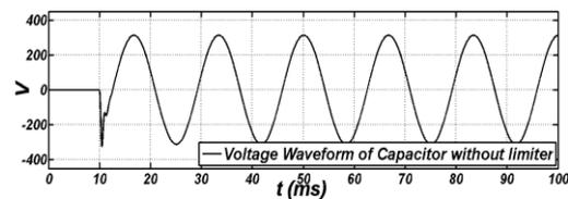
Figure 8. The voltage waveform of capacitor without transient limiter.
