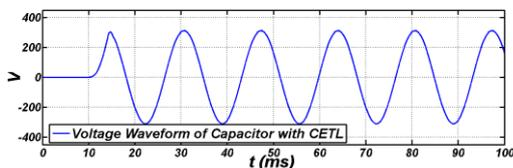
Figure 12. The voltage waveforms of capacitor with limiter and angle 60°.
