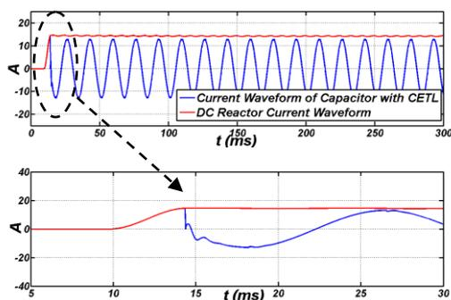
Figure 13. : The current waveforms of capacitor and reactor DC current with the proposed limiter and source angle 60°.
