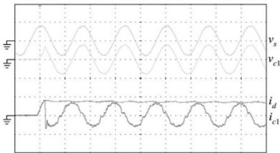
Figure 11. The voltage and current waveforms of capacitor with limiter and angle 60° at the laboratory [12].
