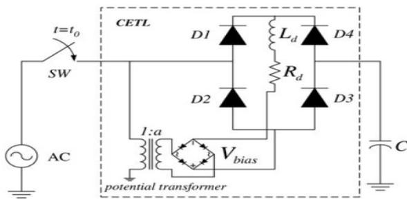
Figure 2. Single-phase circuit diagram of CETL.
