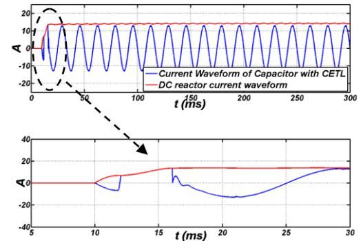
Figure 15. The current waveforms of capacitor and reactor DC current with the proposed limiter and source angle 0°.
