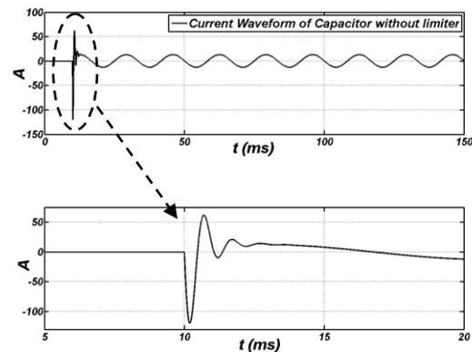
Figure 9. The current waveforms of capacitor without limiter.
