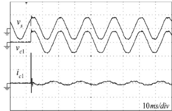
Figure 7. The voltage and current waveforms of capacitor without limiter in the laboratory [12].
