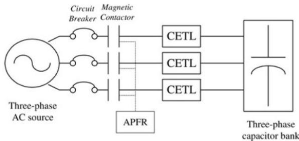
Figure 1. Installation of the CETL in a three-phase distribution system.
