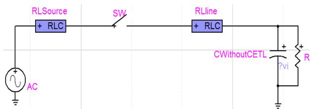
Figure 6. The circuit was simulated using EMTP-RV software without transient limiter.
