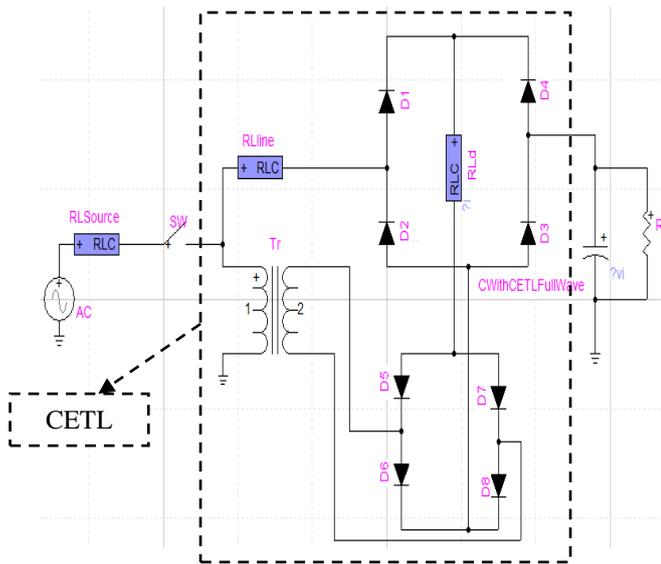
Figure 10. Circuit case study with the proposed limiter.
