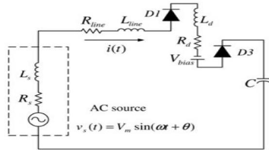
Figure 4. Circuit diagram of CETL in the charging suppressive mode.
