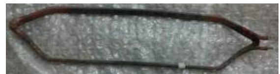
Figure.5. the coil of 6kv generator tested
