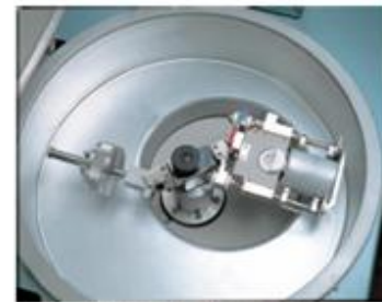
Interior of casting chamber
