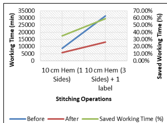
Figure 6. Comparison of time incurred on each stitching operation of the stitching line
