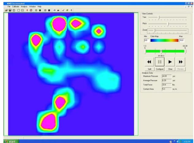
Figure 2. The ForceMap™ system analysis window provides total force and pressure for the entire hand and individual fingers. The analysis
