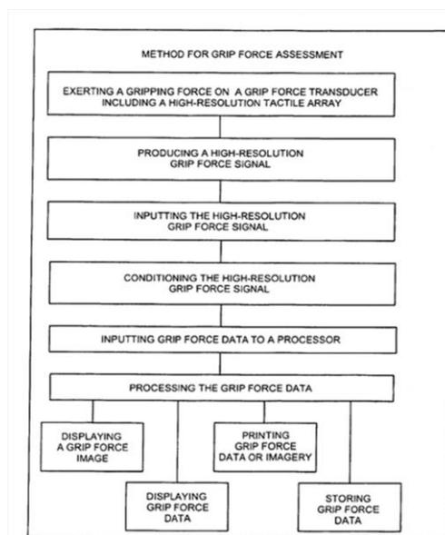
Figure 3. A schematic depicting the steps in involved in the collection and presentation of grip contact force and force distribution via the ForceMap™ system.
