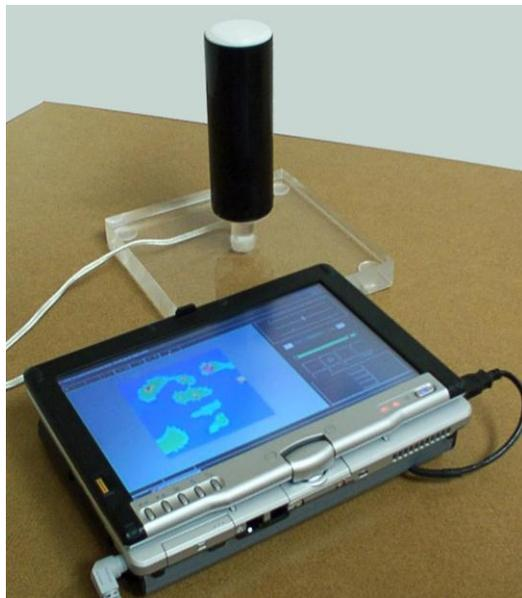
Figure 1. The Hand Grip ForceMap™ System comprised of a high resolution tactile array sensor mounted to a Delrin™ cylinder (grip force transducer) that is interfaced to an amplifier/processor and laptop computer.
