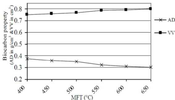
Figure 3. Apparent density (AD) and void volume (VV) of tamarisk biocarbon made under different maximum final temperatures (MFT).
