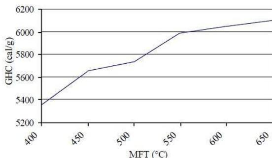
Figure 4. Gross heat of combustion (GHC) of tamarisk biocarbon made under different maximum final temperatures (MFT).
