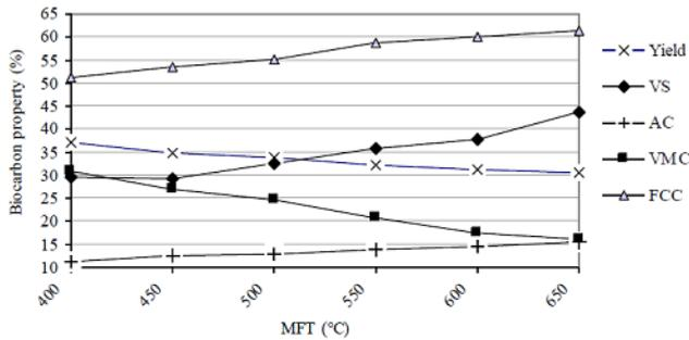
Figure 2. Yield, volumetric shrinkage (VS), ash content (AC), volatile matter content (VMC) and fixed carbon content (FCC) of tamarisk biocarbon made under different maximum final temperatures (MFT).
