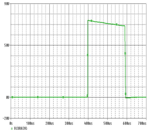
Figure.9.b Simulated drain voltage for the Power MOSFET transistor without self heating effect
