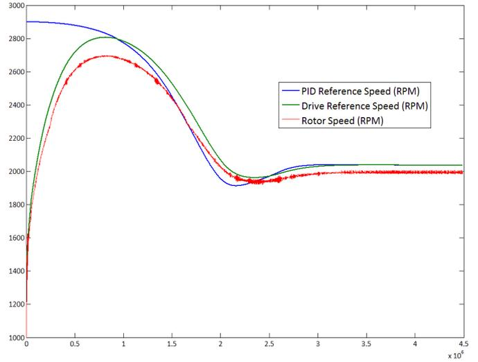
Figure 14. Rotor speed in variable speed strategy
