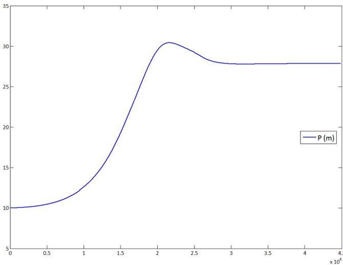
Figure 18. Header pressure in variable speed control strategy
