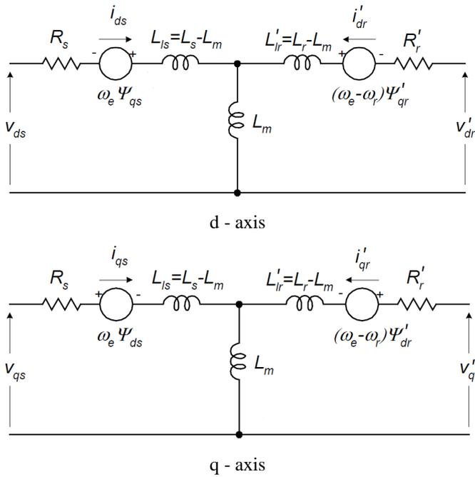
Figure 3. dqo equivalent diagram of induction motor
