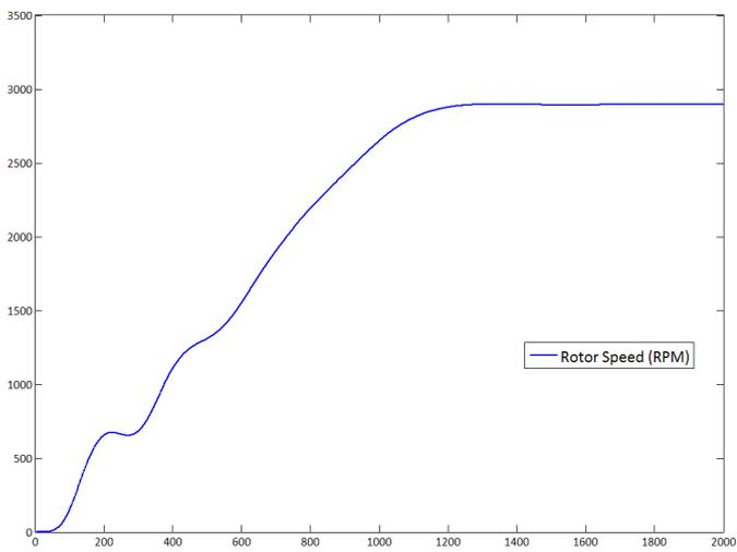
Figure 13. Rotor speed in constant speed strategy
