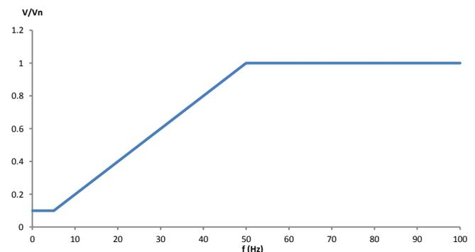
Figure 9. Determining of drive output voltage amplitude in  $V/f = C$
