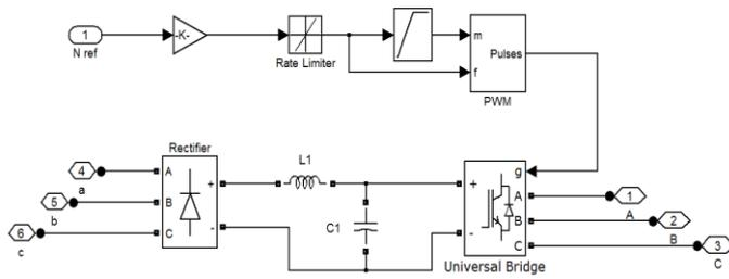
Figure 4. VFD modeling with  $V/f = Cte$
