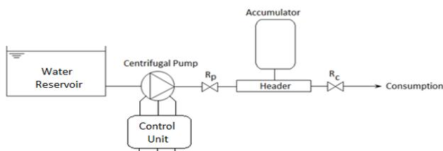
Figure 1. Pumping system set up
