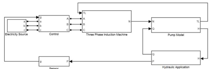
Figure 2. Pumping system modeling in SIMULINK
