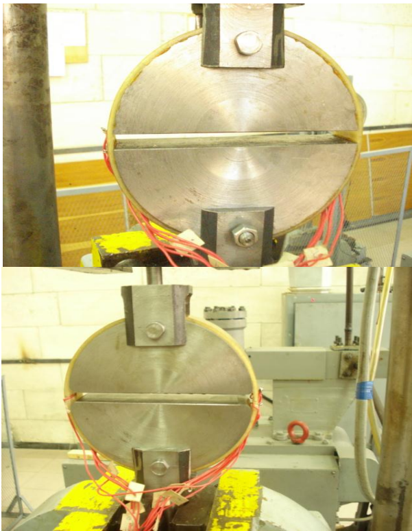
Figure 6 (a, b) Shown the bars, strain gauges and instruments were used in experiment.
