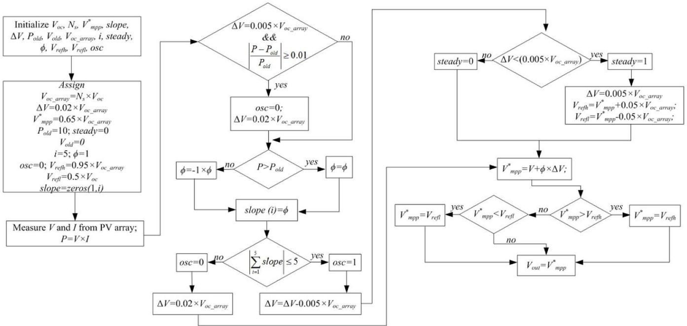
Figure 12. Modified P&O algorithm from [19]
