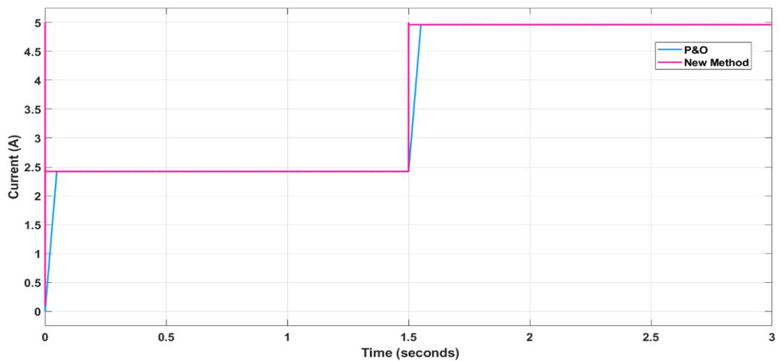
Figure 10. The output current of the new algorithm and the traditional algorithm
