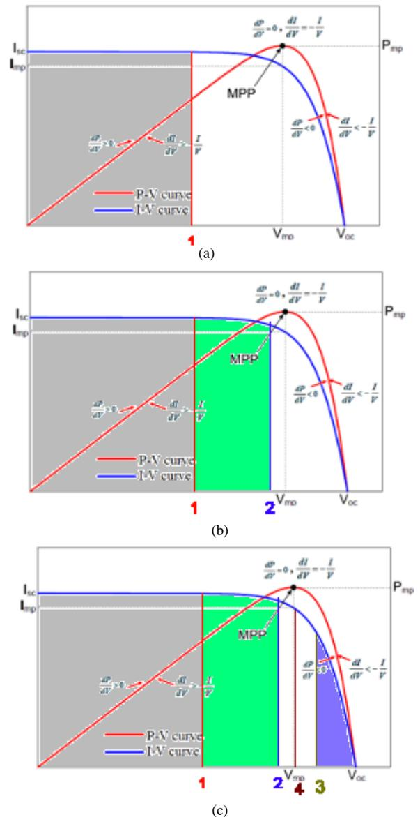
Figure 4. The operating scenario of the proposed method (VOC: the open-circuit voltage, ISC: the short circuit current)
