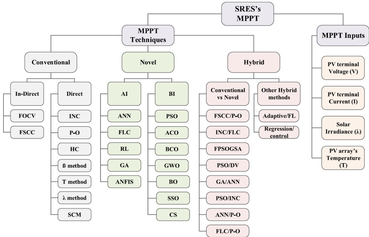
Figure 2. The most MPPT in literature and the control variables [3]
