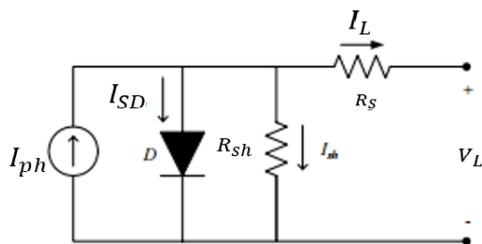
Figure 3. A single diode PV model
