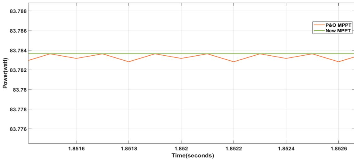
Figure 9. Zooming in of the output power of the new algorithm and the traditional method
