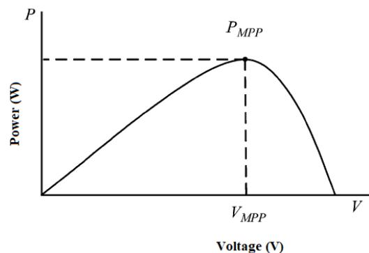
Figure 1. The power to voltage curve of PV panel [3]
