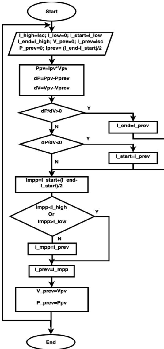
Figure 5. The flowchart of the proposed technique
