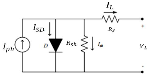
Figure 3. A single diode PV model
