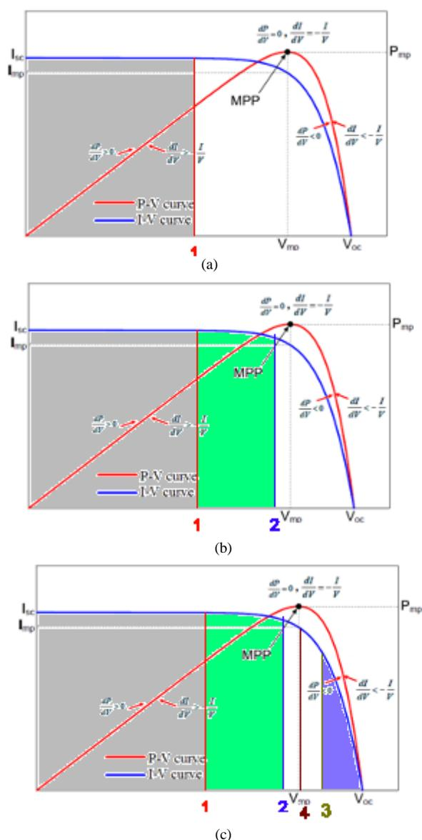
Figure 4. The operating scenario of the proposed method (VOC: the open-circuit voltage, ISC: the short circuit current)
