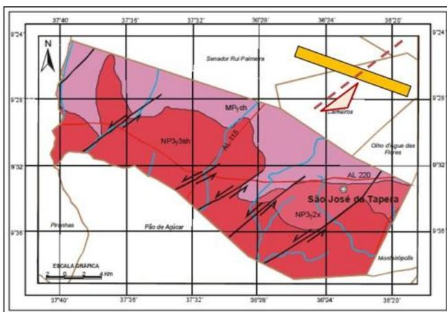
Figure 2. Geological map in the region of the work. Highlight the tunnel direction and the presence of faults in the oblique direction (NE) with a predominant slope for SE. Source: CPRM, 2009.
