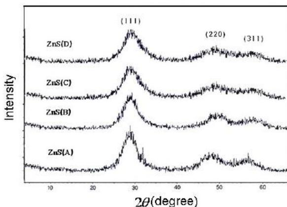
Fig.1 XRD patterns of ZnS nanoparticles with different capping agent molar
