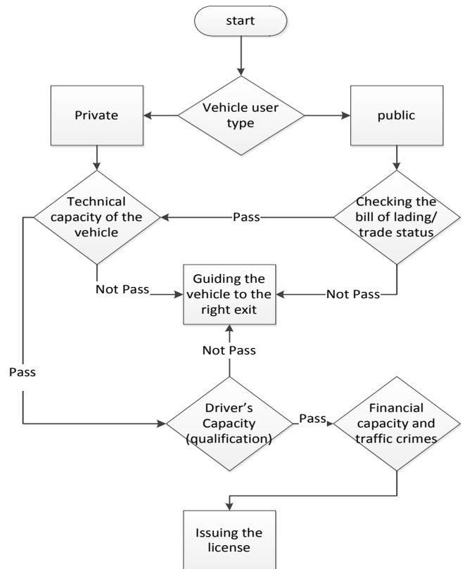
Fig. 7 Mechanism of system
