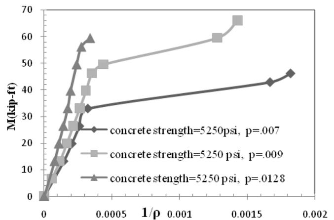
Figure 5: Moment curvature of different steel ratio for fixed concrete strength 5250psi (from experiment)
