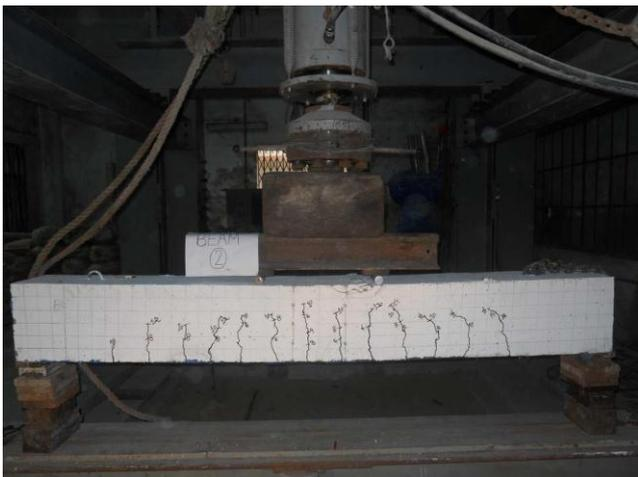
Figure 2: Beam specimen in test frame
