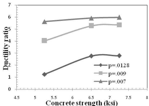
Figure 9: Change in concrete strength with ductility ratio
