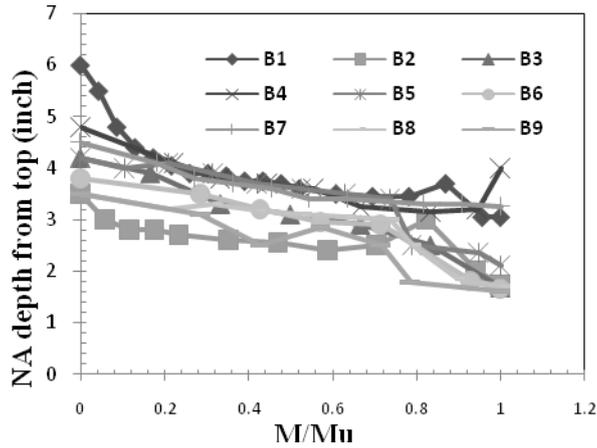
Figure 4: NA depth variation with moment ratio
