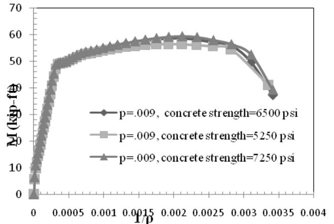
Figure 8: Moment curvature of different concrete strength for fixed steel ratio  $p=0.009$  (from numerical analysis)
