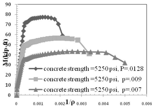
Figure 6: Moment curvature of different steel ratio for fixed concrete strength 5250psi (from numerical analysis)
