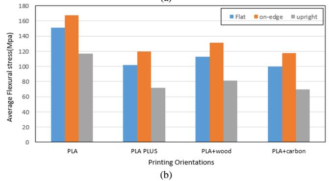
Figure 4. Variation of average flexural strength of FDM specimens of PLA and PLA composites printed with various: (a) layer thickness, (b) printing orientations.
