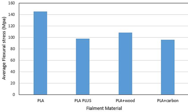
Figure 5. Variation of average flexural strength of FDM specimens of every material with all process parameters variation.
