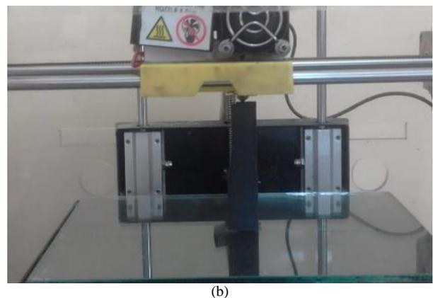
Figure 1. a) The schematic of the Fused Deposition Modeling (FDM) method, b) flexural specimen printed in upright.
