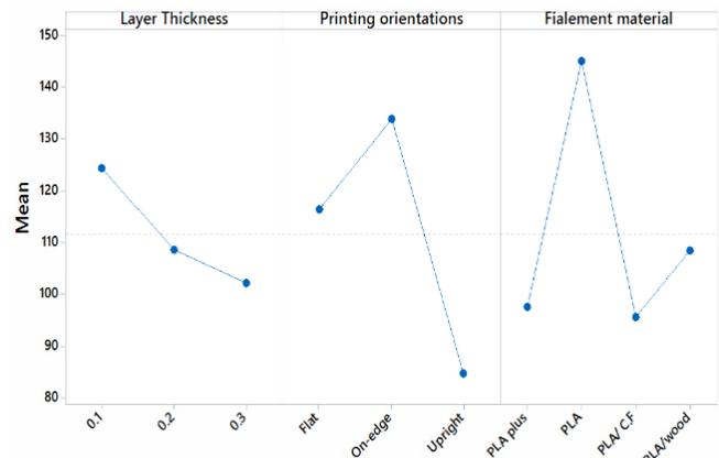
Figure 6. Main Effects plot for Flexural strength.
