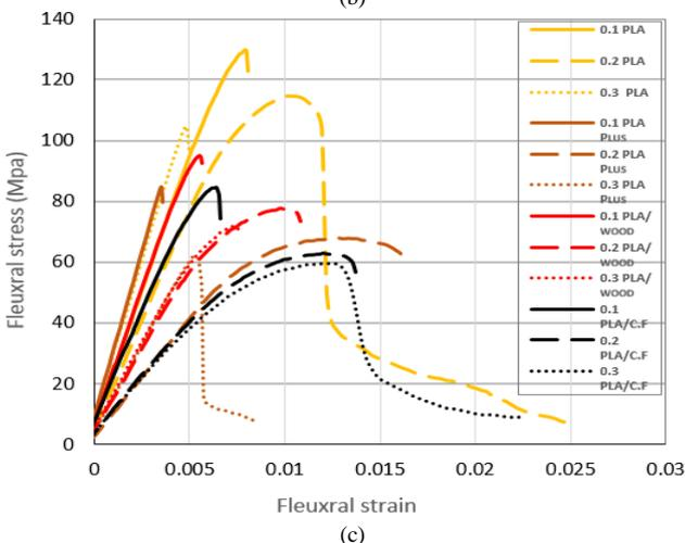
Figure 3. Flexural stress-strain curves of FDM specimens of PLA and PLA composites printed with different layer thickness combinations under different printing orientations: (a) flat, (b) on-edge, (c) upright.
