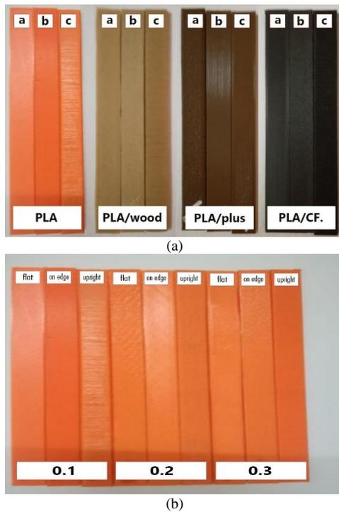
Figure 2. Flexural specimens with a) a-flat, b-on-edge, and c-upright orientation of different materials, b) Virgin PLA with various printing orientations and layer thickness
